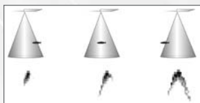
Transducer Cone and Fish Arches
